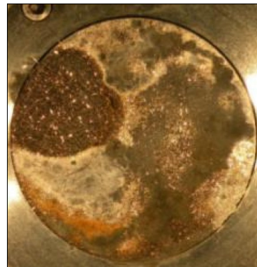
(b) Steel sample from Test 6 without corrosion product layer
