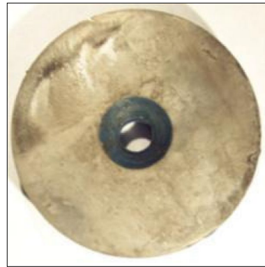
(b) Sample after removal of the corrosion layer
