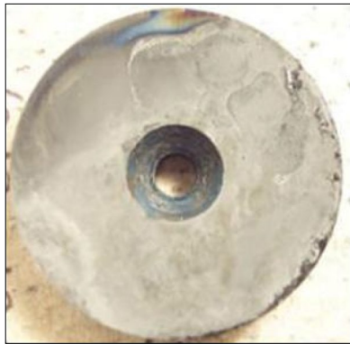
(a) Sample with intact corrosion product layer
