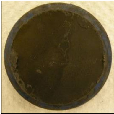
(a) Steel sample with corrosion product layer
