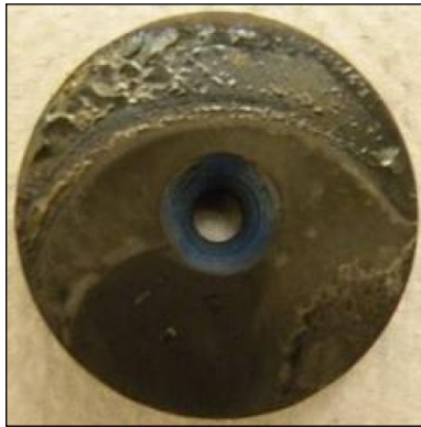
(a) Sample with intact corrosion product layer
